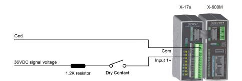
To monitor a DC voltage that is greater than the input rating of the X-17s, a series resistor can be used to reduce the input current.
