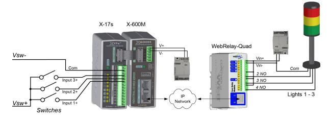
This type of setup allows for switches to be placed far away from the devices they control, and sensors to sound alarms at distant locations.
