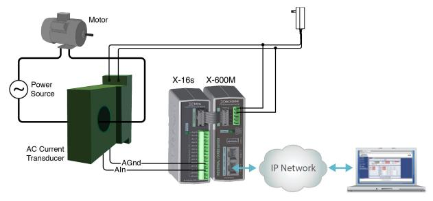
This example uses a current sensor that will measure current up to 20 Amps AC. The sensor produces a linear 0-5VDC output that it can be connected directly to one input of the X-16s analog module. The slope is calculated and entered into the setup pages of the X-600M. The slope calculation is given below:
