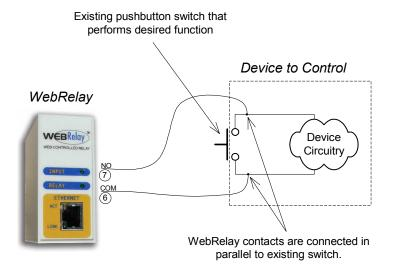
WARNING: Connecting WebRelay<sup>TM</sup> to a device as shown in the illustration above may void the warranty of the device. Additionally, many electrical devices contain dangerously high voltages (even with power disconnected) and should not be opened. The connection illustrated should only be performed by very qualified personnel. Xytronix Research & Design, Inc. will not be responsible or liable for any injury or damage caused by using this connection scheme.
