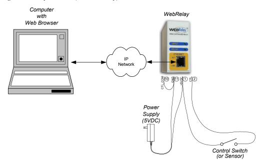
WebRelay<sup>TM</sup> can be used to monitor the status of a device without necessarily controlling anything. Status can be viewed using a web browser or monitored by requesting the XML page. In this example, the internal relay is not being used.
