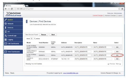
3. In the *Select* column, click the checkboxes of the I/O components you would like to configure and select the **Create Device Widget** option (This will display the status of the I/O on the Dashboard).
