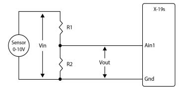
Generally, you can choose a 10K Ohm resistor for R2 and then calculate the value of R1 using the following formula.
