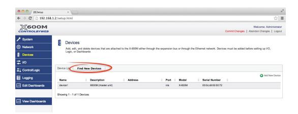
2. In this example we are going to add an X-19s expansion module. Click the Add button for the X-19s.
