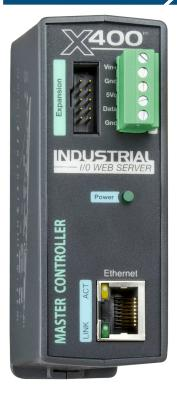
The X-400<sup>™</sup> is a powerful web-enabled industrial I/O controller with advanced logic and modular expansion capabilities.
