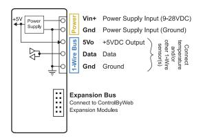
**Warning:** The maximum number of attached expansion modules is determined by power supply voltage and current, and type of modules attached. For some installations, additional power supplies and expansion bus power injectors may be required.
