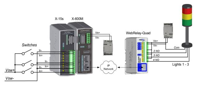
This type of setup allows for switches to be placed far away from the devices they control, and sensors to sound alarms at distant locations.
