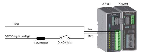
Each digital input has an internal 3K ohm resistor. The forward voltage drop of the photo-coupler is approximately 1.2V and works well with an input current of 9mA. Use the following formula to determine the resistor value needed for other voltage ranges:
